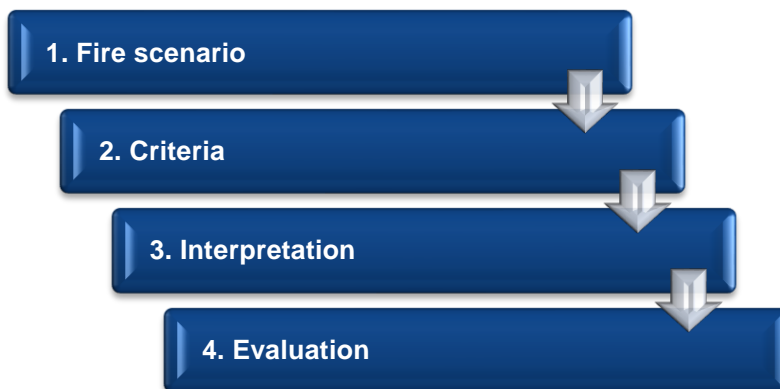
Fig. 2. Process of evaluation of construction products in terms of fire safety according to CEN procedures based on [16, 17]
