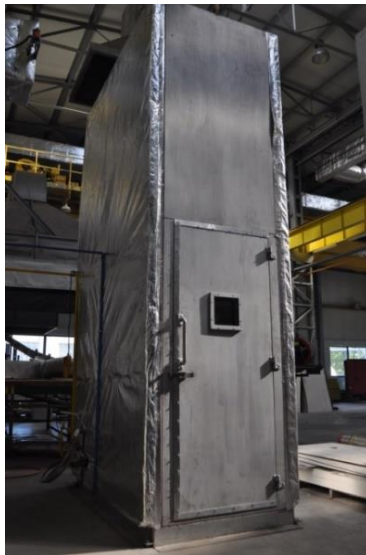
Fig. 6. External view of EN 50399 standard test chamber at the accredited ITB Fire Testing Laboratory in Pionki, Poland
