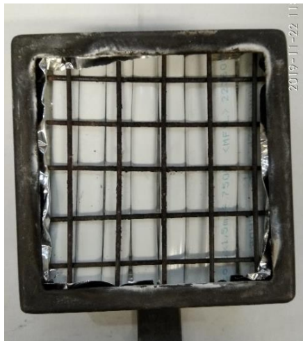
Fig. 22. PVC cable specimen secured by steel grid
